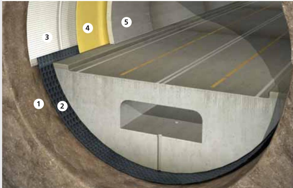
The drainage capacity of Platon P 20 is many times higher than that of Platon Tunnel Membrane, providing even more security. Thanks to the volume of the air gap, 14 l/m<sup>2</sup>, P20 offers high drainage capacity to deal with higher volume or even extreme volume water ingress.
