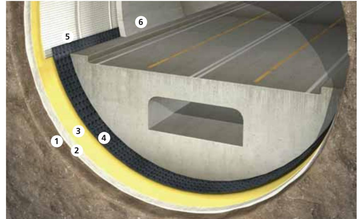
Platon P20 will create a space for grouting beneath the foundation segment and allow a good flow of grout.
